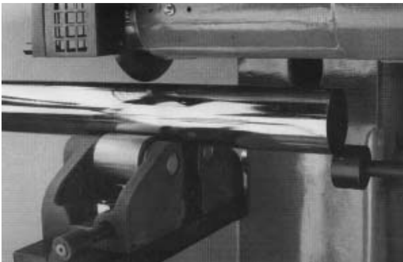
Pipe cutting using a rotary cut-off machine
