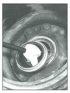
Removing hub oil seals slows down routine brake jobs. Prying or driving them out is time consuming and bearings are often damaged in the process.
