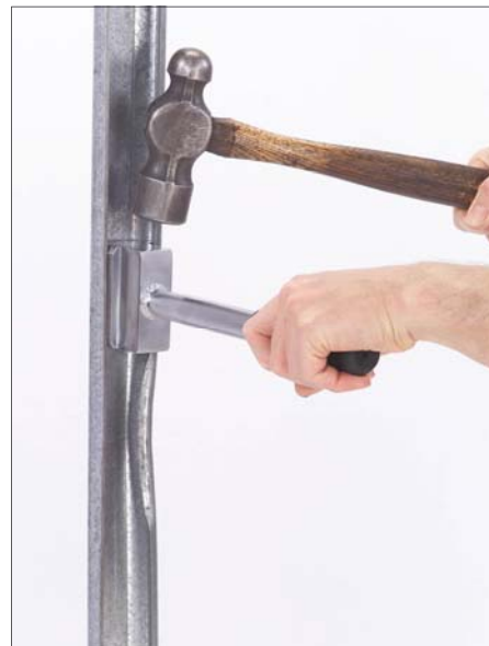
Hammer it through crushed track!
